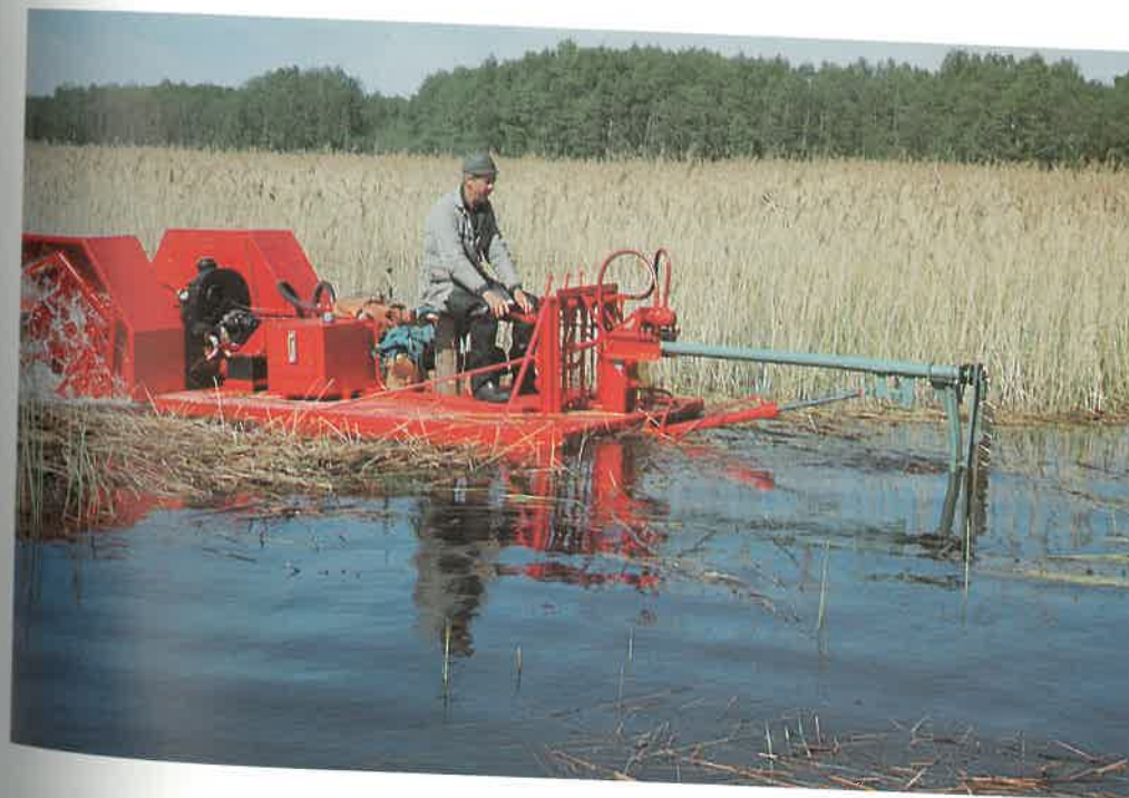
Figure 3. Pontoon machine equipped with horizontal and vertical cutting bars. Constructor Emil Cronqvist. Lake Hornborga, Sweden, 1969. Photo: Sven Björk.
