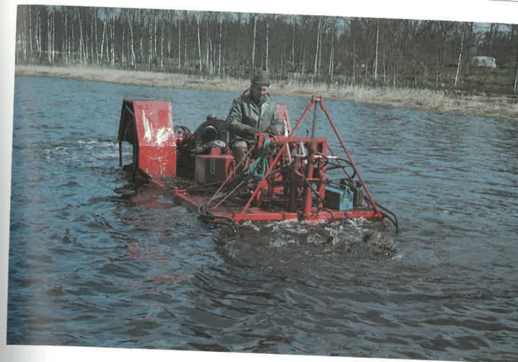
Figure 2. Pontoon machine equipped with rotavator for treatment of roots and rhizomes of aquatic macrophytes. Constructor Emil Cronqvist. Lake Långasjön, Sweden, 1972. Photo: Sven Björk.
