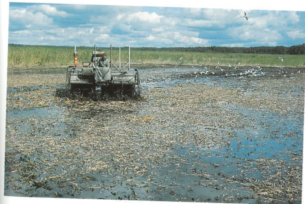
Figure 4. Lake Hornborga. Prototype of rotavator for removal of the stubble mat and rhizome layer of Phragmites . The slowly moving knives cut the rhizomes in long, easily floating pieces. Photo: Sven Björk 1972.
