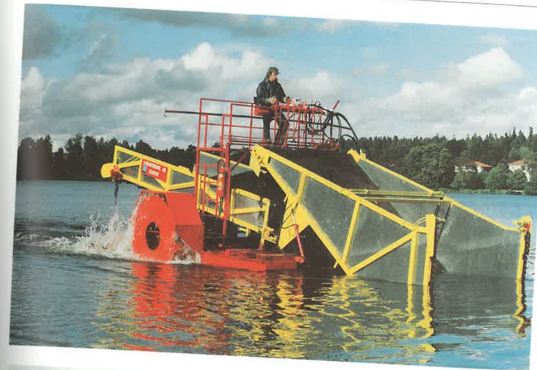
Figure 2. Pontoon harvester Limno-Combine with one horizontal and two vertical cutting bars (above). Automatic unloading of cut plant material (below). Constructor: Emil Cronqvist. Lake Magelungen, Stockholm, 1993. Photo: Stefan Cronqvist.
