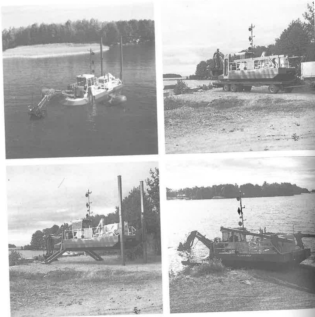
Figure 4. Multipurpose dredger, type Länne Watermaster. Constructor Länne Engineering, Finland. The dredger is easily transported on a lorry and capable of loading and unloading itself as well as launching itself into wetlands and lakes. By courtesy of Länne Engineering.
