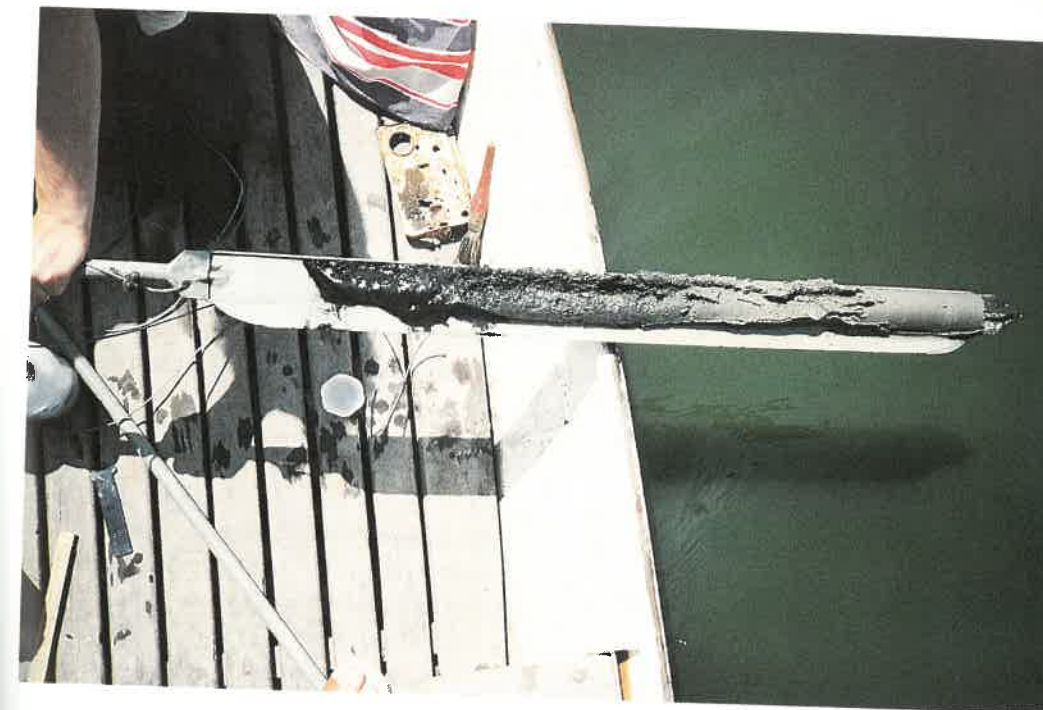
Figure 4. Sediment core with distinctive grey and black layers of sediment.
